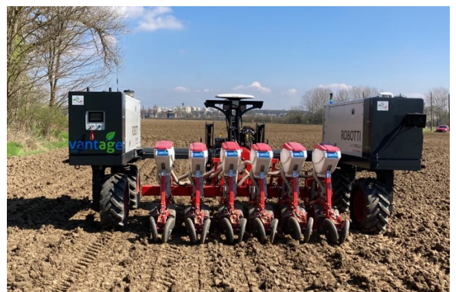
Figure 3-5: 5G-enabled Smart Agriculture Robot Conducting Weeding & Seeding Activity
