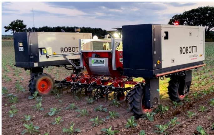
Figure 3-5: 5G-enabled Smart Agriculture Robot Conducting Weeding & Seeding Activity
